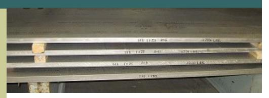
Delivering exceptional strength at high temperatures, alloy 230 plate is a popular alternative to stainless steel and nickel-based alloys. 230 is composed of nickel, chromium, tungsten and molybdenum.
